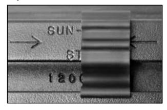
If your vehicle has a sunroof, it will have crossrail stop tabs placed in the siderails. These tabs prevent you from moving the crossrails past the opening of the sunroof and loading cargo too far forward. Cargo loaded too far forward could fall onto the sunroof and into the passenger compartment. Loading cargo too far forward could also cause the OnStar and navigation system (if equipped) to function improperly or not at all.
